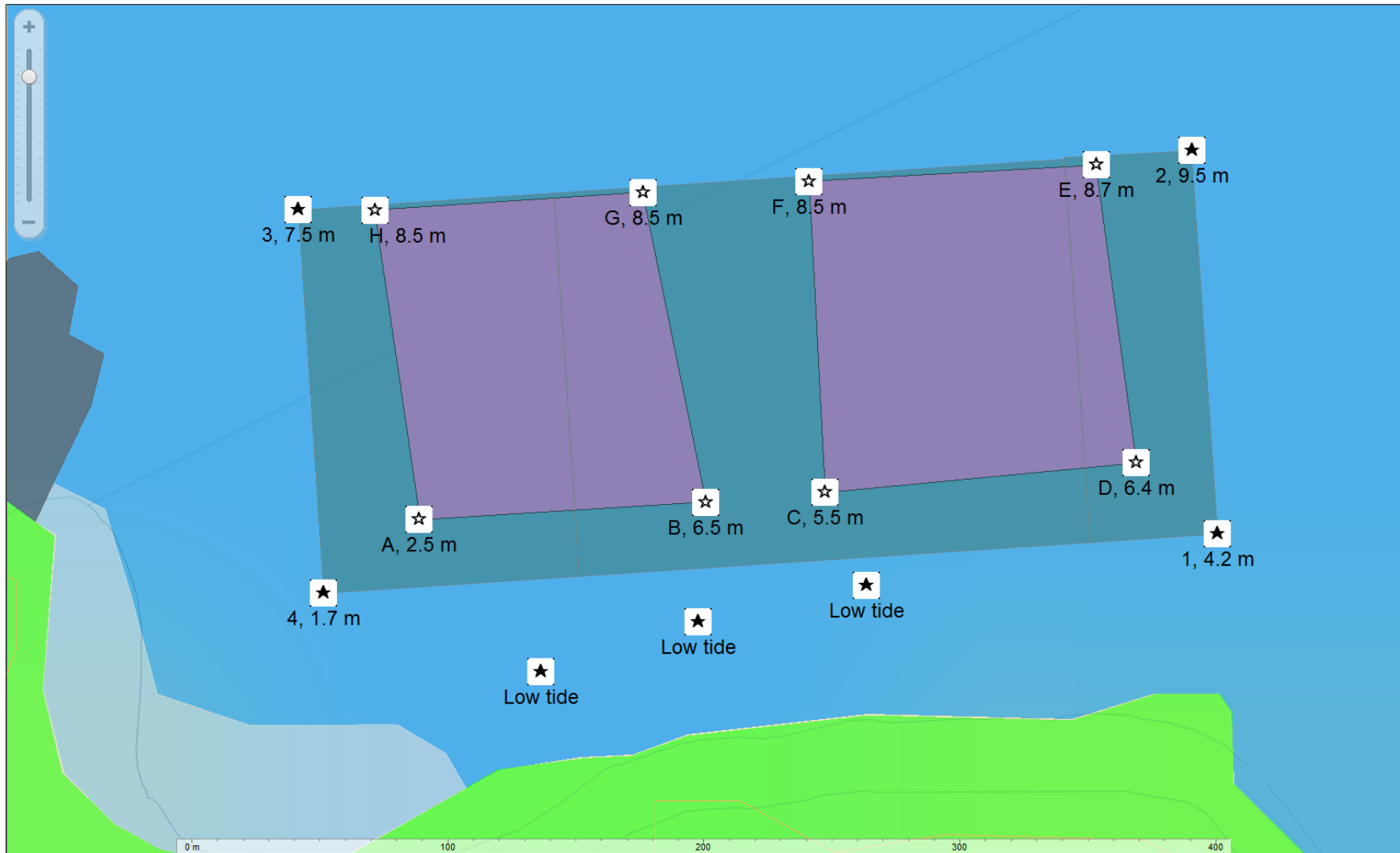
Figure 3. Depths of the consent area (teal), and existing surface structures (pink). Low tide positions are also plotted.
