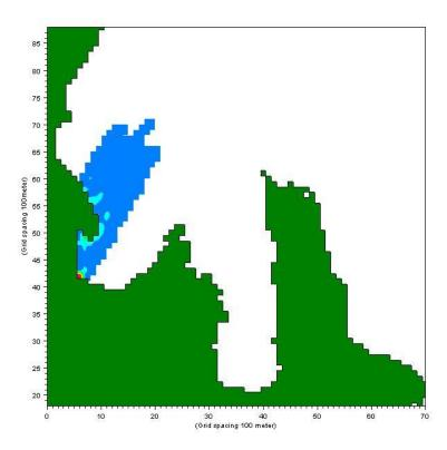
Figure A4.4 Simulation under southwest winds from release point in the Port of Wellington.
