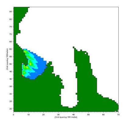
Figure A4.5 Simulation under northwest winds from release point in the Port of Wellington.
